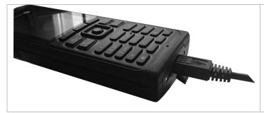
Plug the USB cable into the USB port of your phone. The other end of the USB cable can be plugged into the AC/DC adaptor or into a computer USB port.
